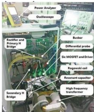
Fig. 13, the prototype of dual active H-bridge
